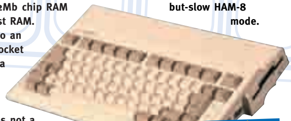
The A600 may have been smaller and cuter than the A500, but it was also less expandable
